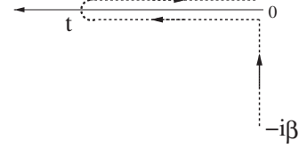
FIG. 1. Kadanoff-Baym-Keldysh contour, which starts at time 0 on the first branch, runs up to time t=t_* then back from t_* to t=0 and finally along the imaginary axis from t=0 to t=-i\beta .
